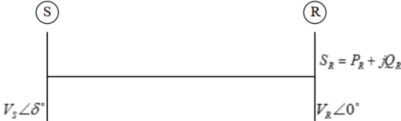
FIG.- TRANSMISSION LINE POWER FLOW
